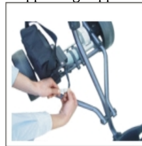
Connect battery to the Power cord on the cart
