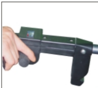
Turn the accelerator knob to open the power
